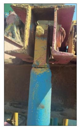
Figure 9. Deformation and wear of the connecting rod-traverse connection
