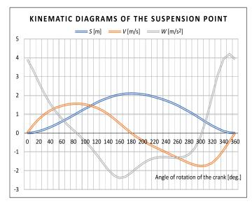
**Figure 4.** Typical kinematic diagrams of the suspension point where *S*, *V*, *W* are the displacement [m], velocity [m/s] and acceleration  $[m/s^2]$  of the suspension point
