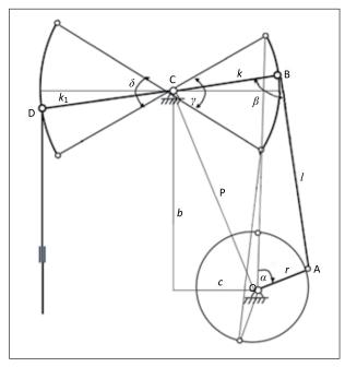
**Figure 3.** Kinematic diagram of the transforming mechanism – pump jack:  $k_1$ , k – front and rear shoulders of the balancer; l – the length of the connecting rod; r – the length of the wheel arm; b, c – coordinates of O support; p – polar distance;  $\alpha$  – rotation angle of the wheel arm;  $\beta$  – pressure angle between the balancer and the connecting rod;  $\delta$ ,  $\gamma$  – turning angles of the front and rear shoulders of the balancer; D – suspension point
