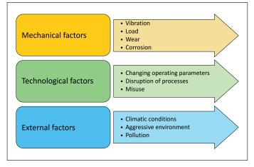
**Figure 1.** Classification of factors influencing the aging process of a pump jack
