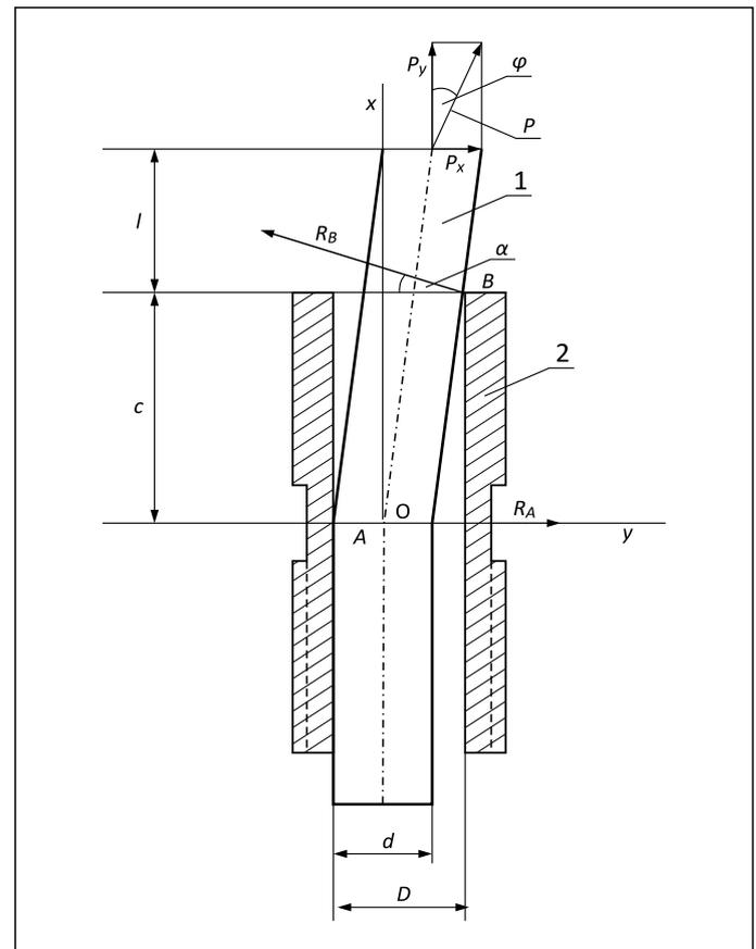
**Figure 1.** Scheme of determining the friction force between the draw rod and the guide: 1 – draw rod; 2 – guide
