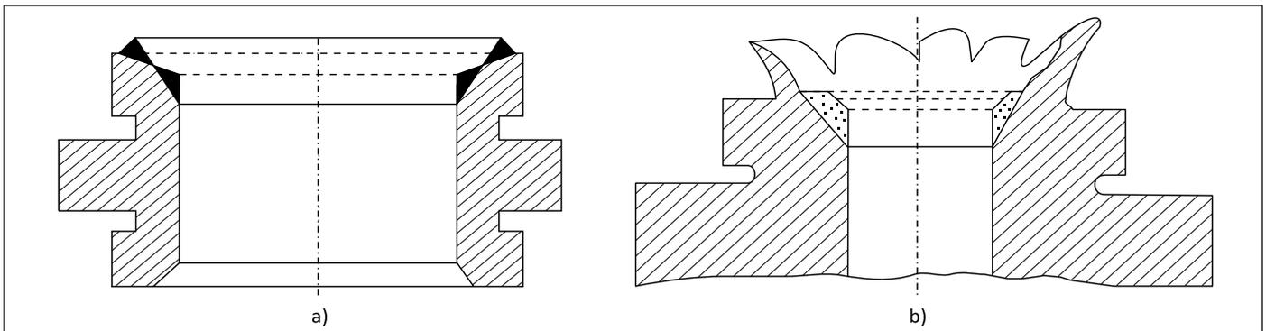
**Figure 6.** A saddle with a deformed chamfer: a) a saddle with an enlarged chamfer as a result of deformation, b) protrusions formed in the facade as a result of deformation
