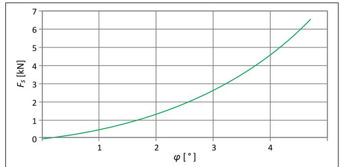
**Figure 2.** Dependence of friction force between draw rod and guide at  $\varphi$  angle
