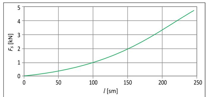
**Figure 3.** The graph of the dependence of the friction force between the draw rod and the guide on the travel path of the plunger when  $\varphi = 3^\circ$
