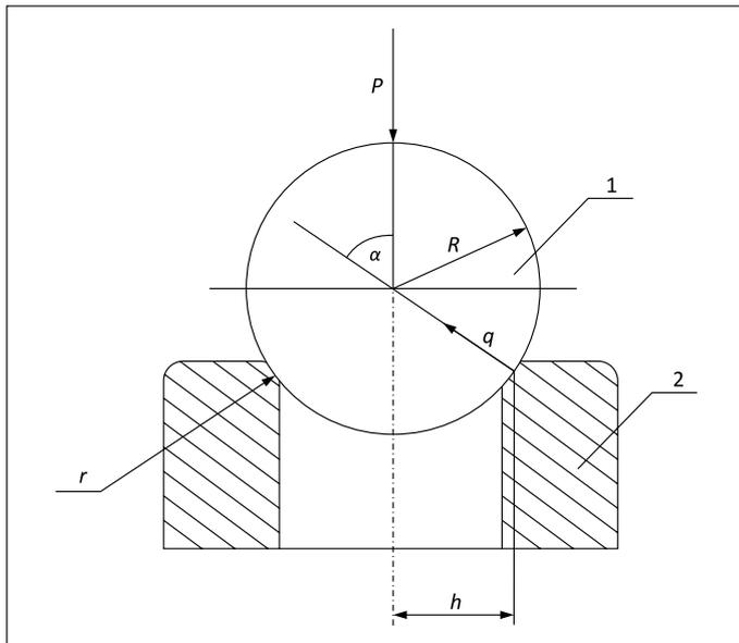
Figure 4. Calculation scheme of the “Ball-saddle” pair: 1 – sphere; 2 – saddle
