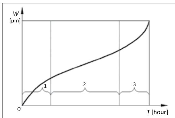
**Figure 1.** Wear curve of sealing parts of machinery and equipment under the action of friction according to the IT diagram; 1 – running-in period, 2 – period of normal operation, 3 – period of intensive wear,  $W$  – value of wear [microns],  $T$  – the duration of work [hour]
