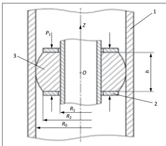
**Figure 3.** Scheme of deformation of the sealing element: 1 – support sealing, 2 – support washer, 3 – sealing for rubber
