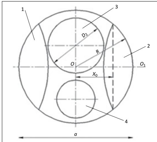
**Figure 2.** Scheme for determining the geometric characteristics of the elastic element of the packer seal; 1, 2 – volumes extracted from the elastic element, 3, 4 – eccentric holes
