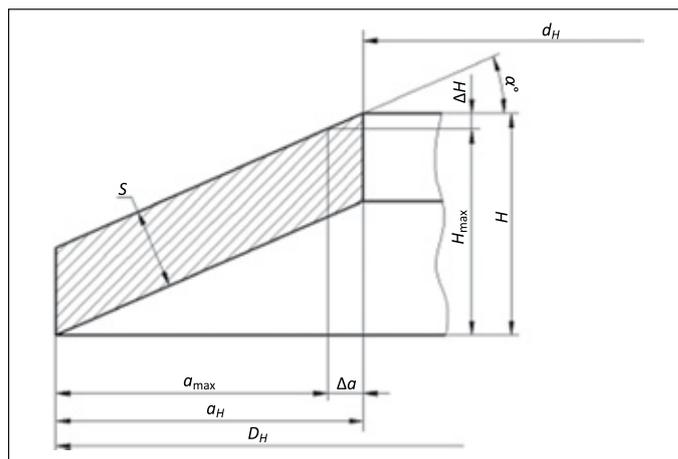
**Figure 6.** Scheme for calculating spring height deviations
