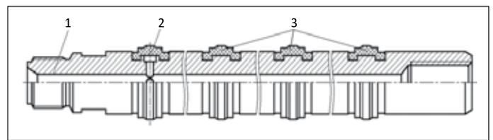
**Figure 4.** The design of the sleeve plungers of borehole pumps; 1 – plunger body; 2 – rubber ring, 3 – swelling rubber rings
