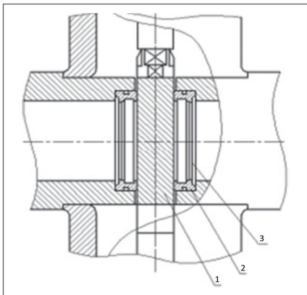
**Figure 5.** Valve operating unit; 1 – seat, 2 – gate, 3 – disk spring
