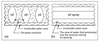
**Figure 3.** Scheme of the movement of oil and water through porous channels with mixed (emulsion) (a) and jet (b) flow structures
