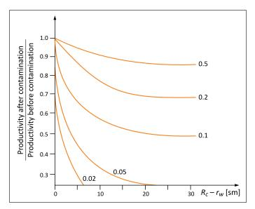
Figure 2. Decrease in well productivity depending on the depth of damage
