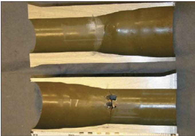
**Figure 3.** Flushing hole and fatigue crack in internal failure (Zamani et al., 2016)
