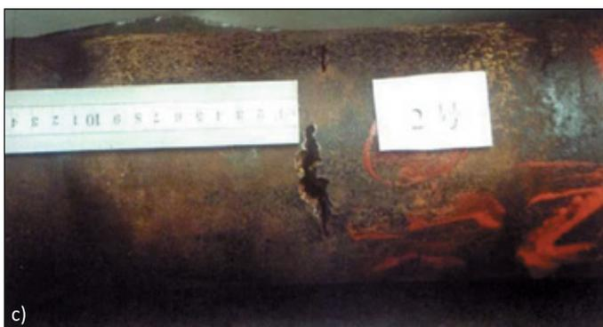
**Figure 1.** Morphology of corrosion ulcers on the inner surface of the flushing hole (a) and cracks arising from corrosion ulcers near the end of the internal narrowing (b), as well as flushing on the drill pipe (c) (Lu et al., 2005; Lukin et al., 2020)
