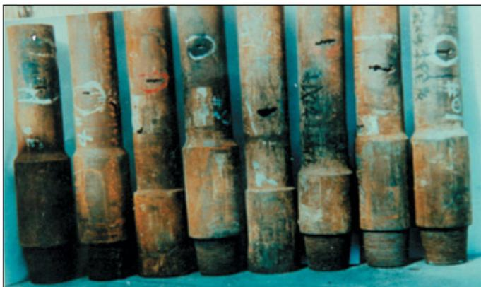
**Figure 4.** Flushing holes of the drill pipe in the transition zone (Liu et al., 2011)
