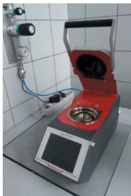
Fig. 2. RapidOxy 100 instrument for the oxidation stability determination (photo INiG – PIB)
