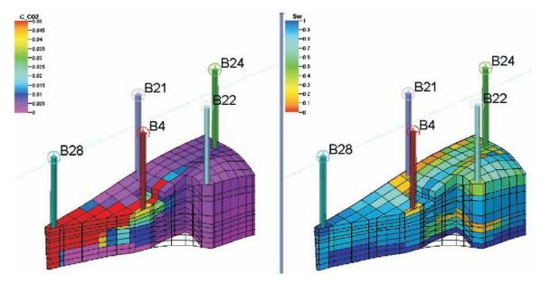
Fig. 12. CO<sub>2</sub> (left panel) and water (right panel) distribution in the Borzęcin structure
