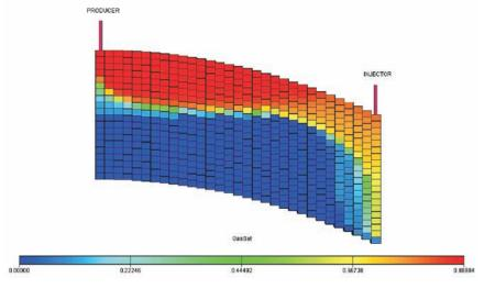
Fig. 6. Gas saturation between injector and producer
